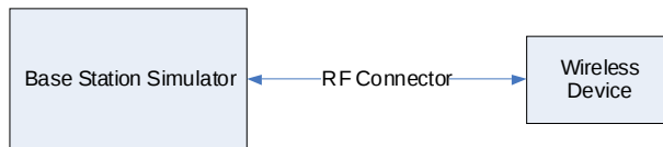
Figure 13-1 Power Measurement Setup
