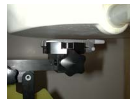
Figure 14.10 Body SAR Test Setup -- w/o Holster --
