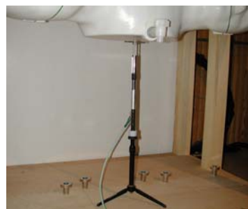
Figure 12.1 Dipole Validation Test Setup
