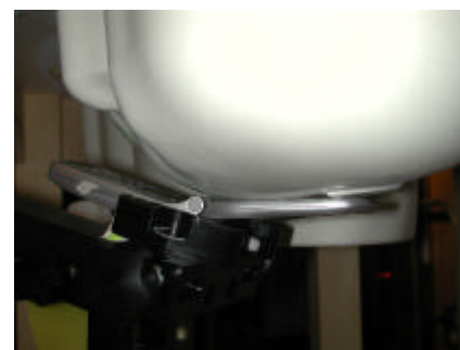
Figure 15.3 Left Head SAR Test Setup -- Cheek / Touch Position --
