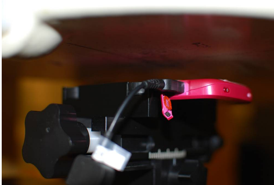
SAR Test Setup Photo 5 – Body Worn at 1.5 cm
