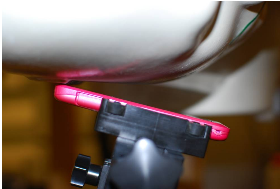
SAR Test Setup Photo 2 – Right Tilt
