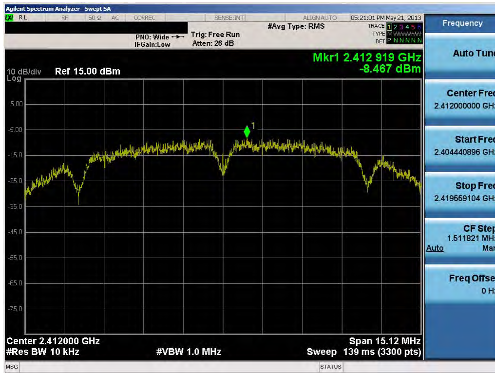
Plot 6-13. Power Spectral Density Plot (802.11b – Ch. 1)
