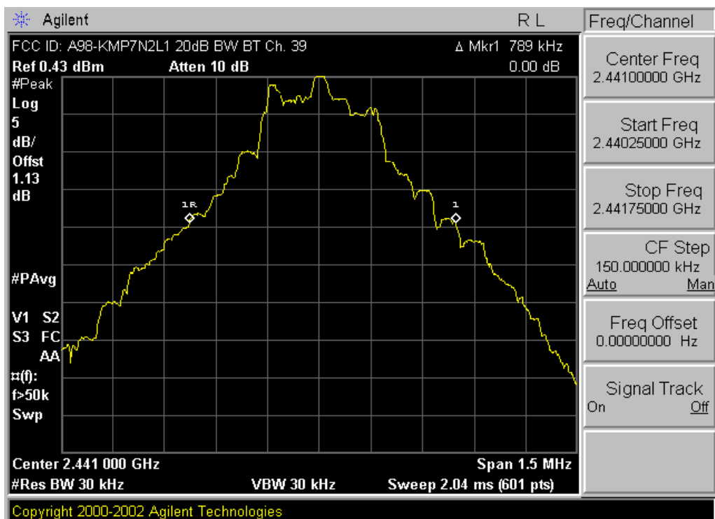
Plot 6-2. 20dB Bandwidth Plot (Bluetooth – Ch. 39)
