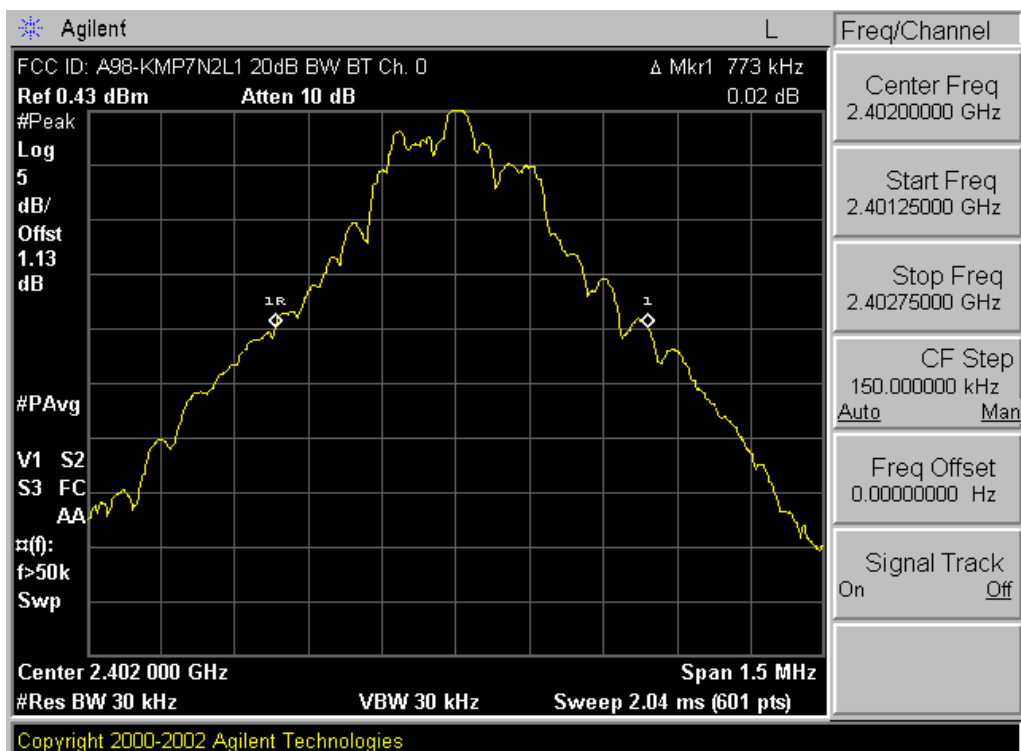
Plot 6-1. 20dB Bandwidth Plot (Bluetooth – Ch. 0)
