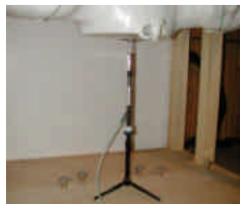
Figure 12.1 Dipole Validation Test Setup
