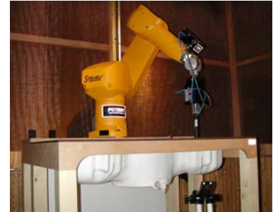
Figure 6.1 DASY3 Test System
