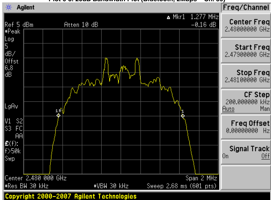
Plot 6-6. 20dB Bandwidth Plot (Bluetooth, 2Mbps – Ch. 78)
