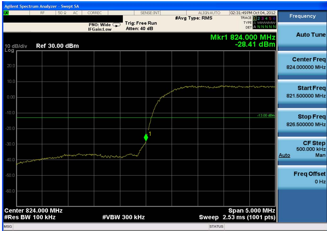
Plot 7-5. Band Edge Plot (Cellular WCDMA Mode – Ch. 4132)
