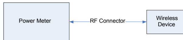
Figure 14-2 Power Measurement Setup
