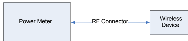
Figure 14-2 Power Measurement Setup
