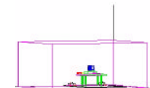
Figure 3-1. Shielded Enclosure Line-Conducted Test Facility
