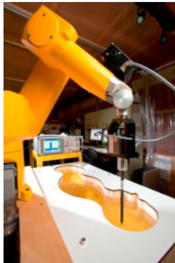
Figure 3-2 DASY4 SAR Measurement System
