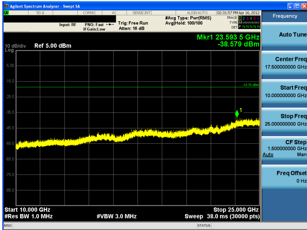
Plot 6-12. Conducted Spurious Plot (Bluetooth LE – Ch. 17)
