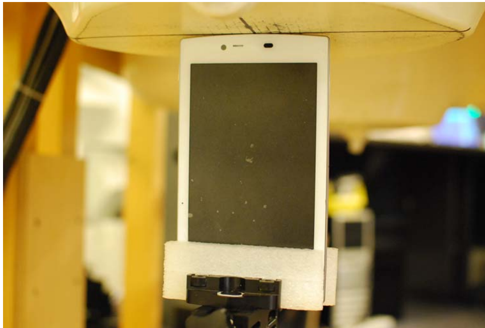
SAR Test Setup Photo 6: Top Edge at 0.0 cm
