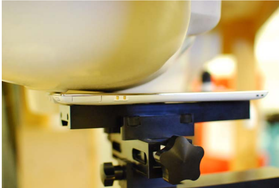
SAR Test Setup Photo 1: Right Touch
