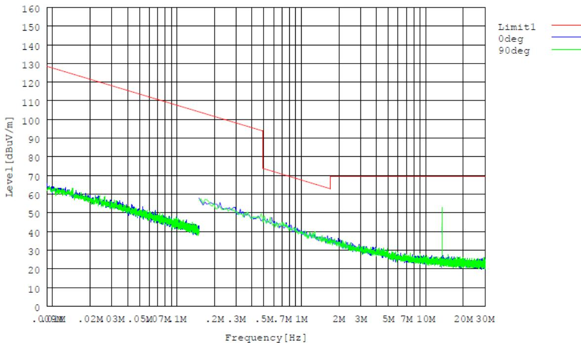
Note : 13.56 MHz is a Tx carrier. This is not spurious emission from EUT.
