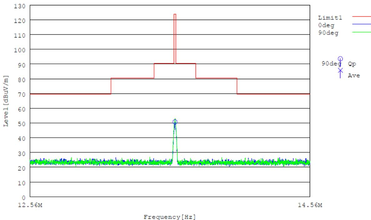
§15.225(d) Harmonics and spurious emission between 9 kHz to 30MHz (refer 15.209 and 15.205)
