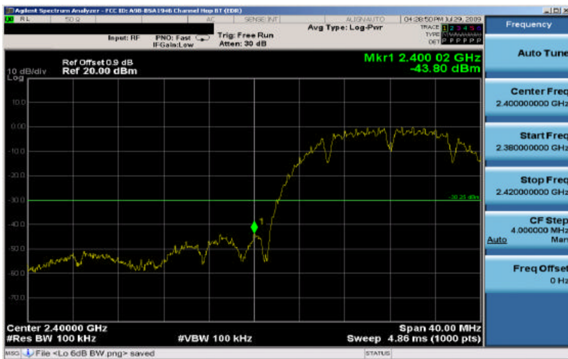
Plot 6-13. Band Edge Plot (802.11b – Ch. 1)
