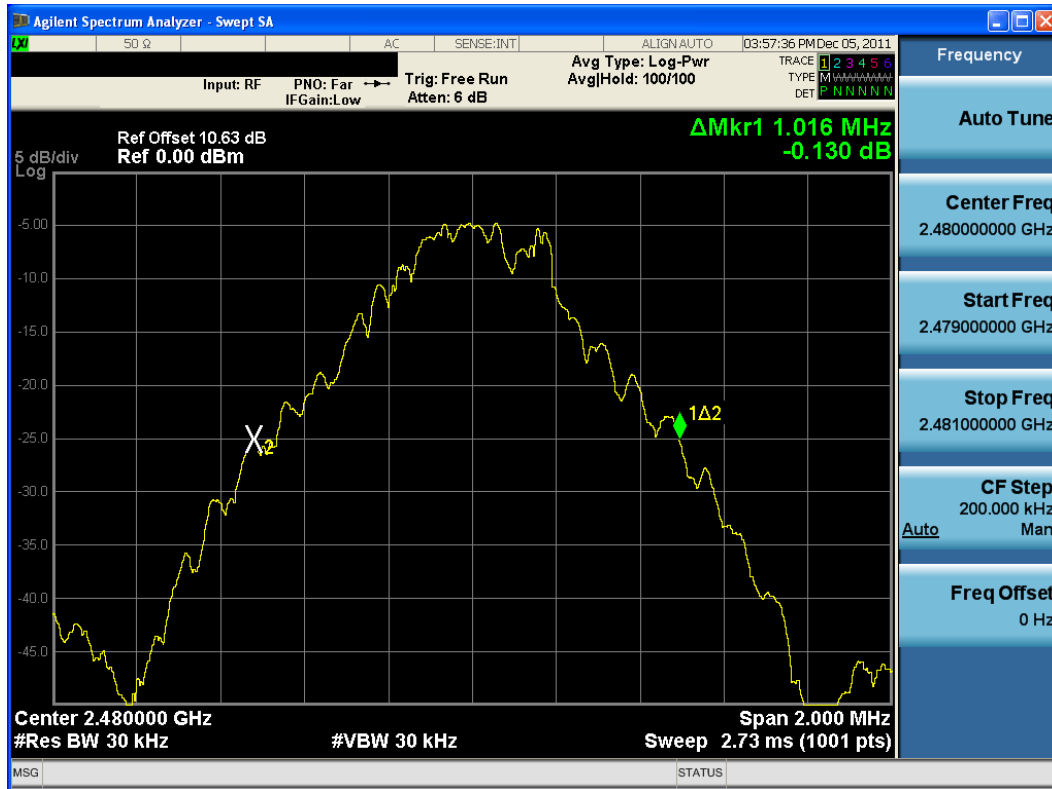
Plot 6-3. 20dB Bandwidth Plot (Bluetooth, 1Mbps – Ch. 78)
