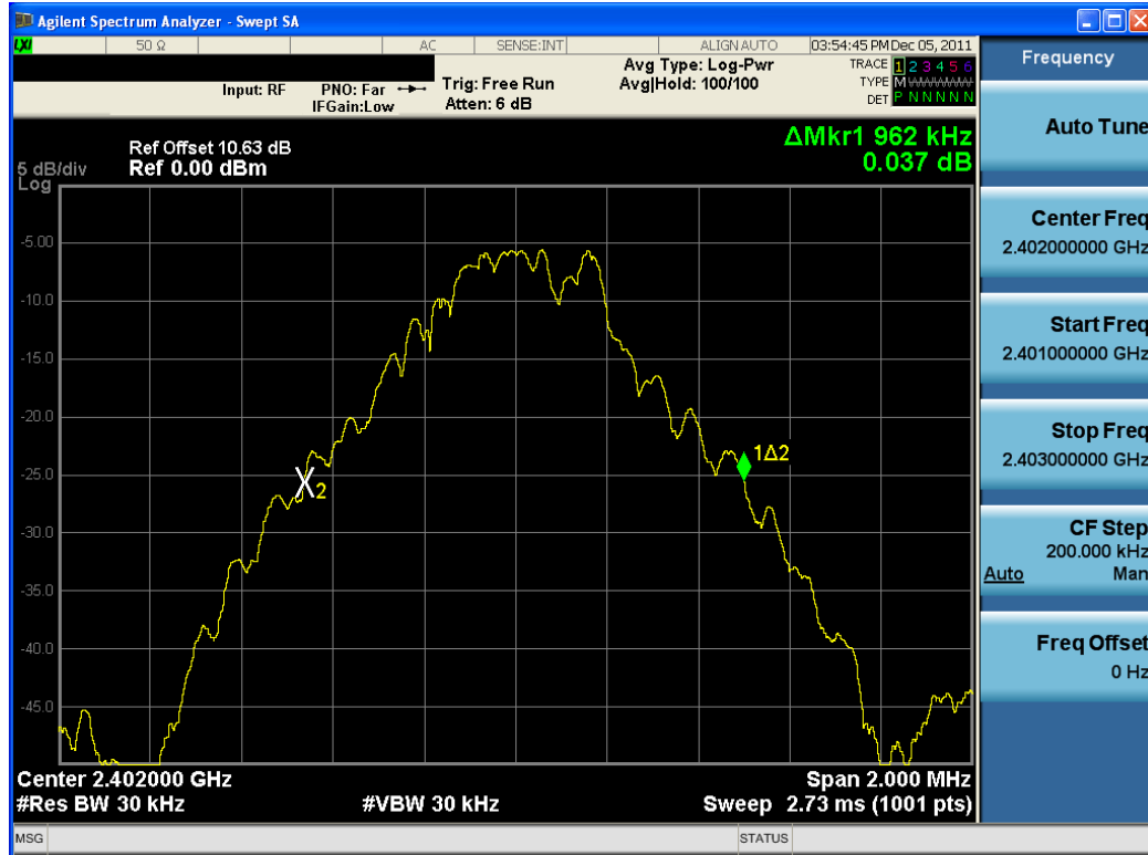
Plot 6-1. 20dB Bandwidth Plot (Bluetooth, 1Mbps – Ch. 0)
