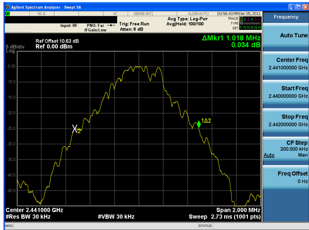
Plot 6-2. 20dB Bandwidth Plot (Bluetooth, 1Mbps – Ch. 39)
