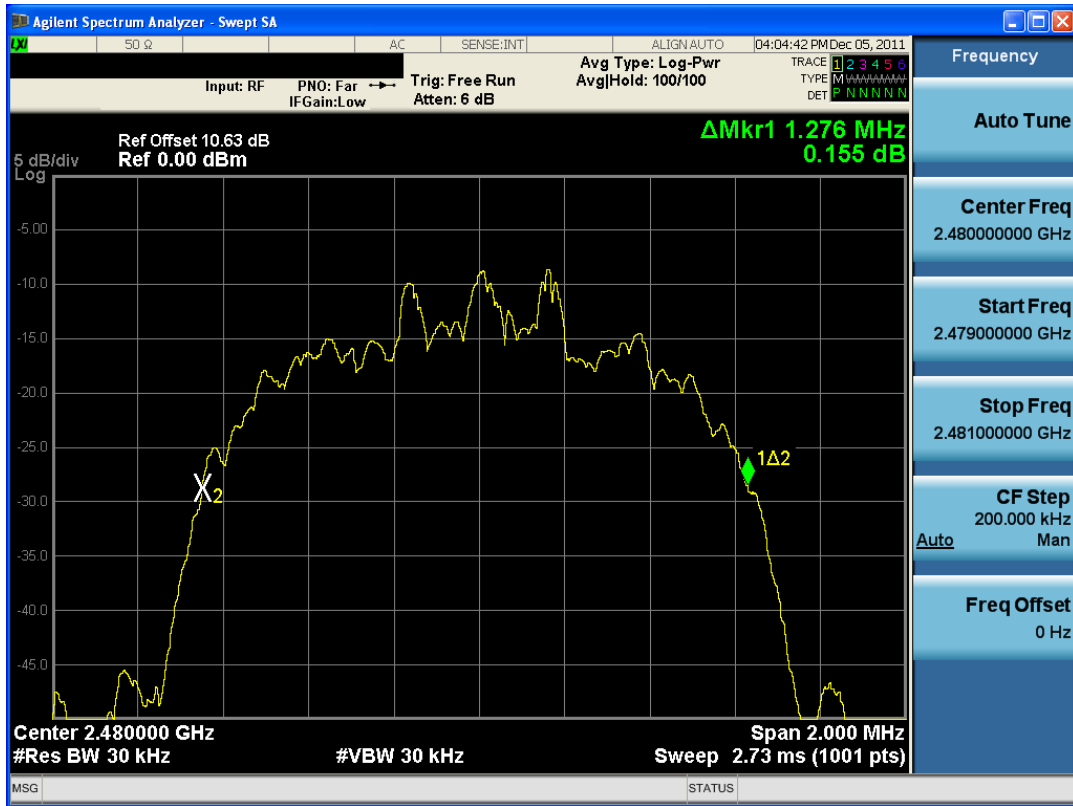
Plot 6-9. 20dB Bandwidth Plot (Bluetooth, 3Mbps – Ch. 78)
