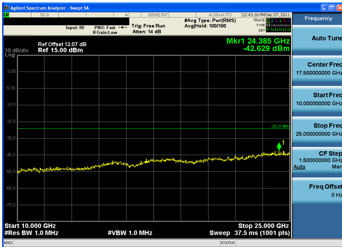
Plot 6-26. Conducted Spurious Plot (802.11b – Ch. 1)
