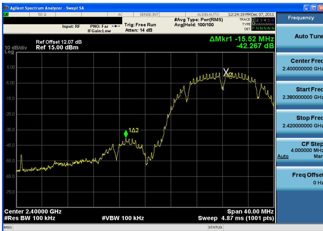
Plot 6-19. Band Edge Plot (802.11b – Ch. 1)
