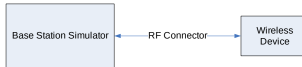
Figure 12-1 Power Measurement Setup
