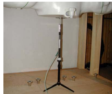
Figure 12-2 System Verification Setup Photo
