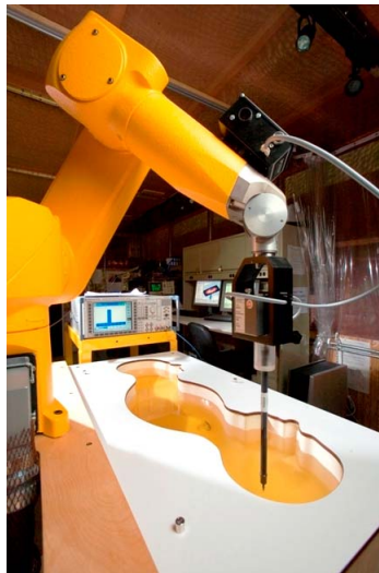
Figure 3-2 DASY4 SAR Measurement System
