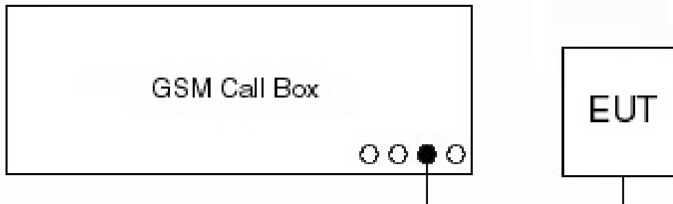
Figure 6-1. GSM Conducted Power Test Setup Diagram
