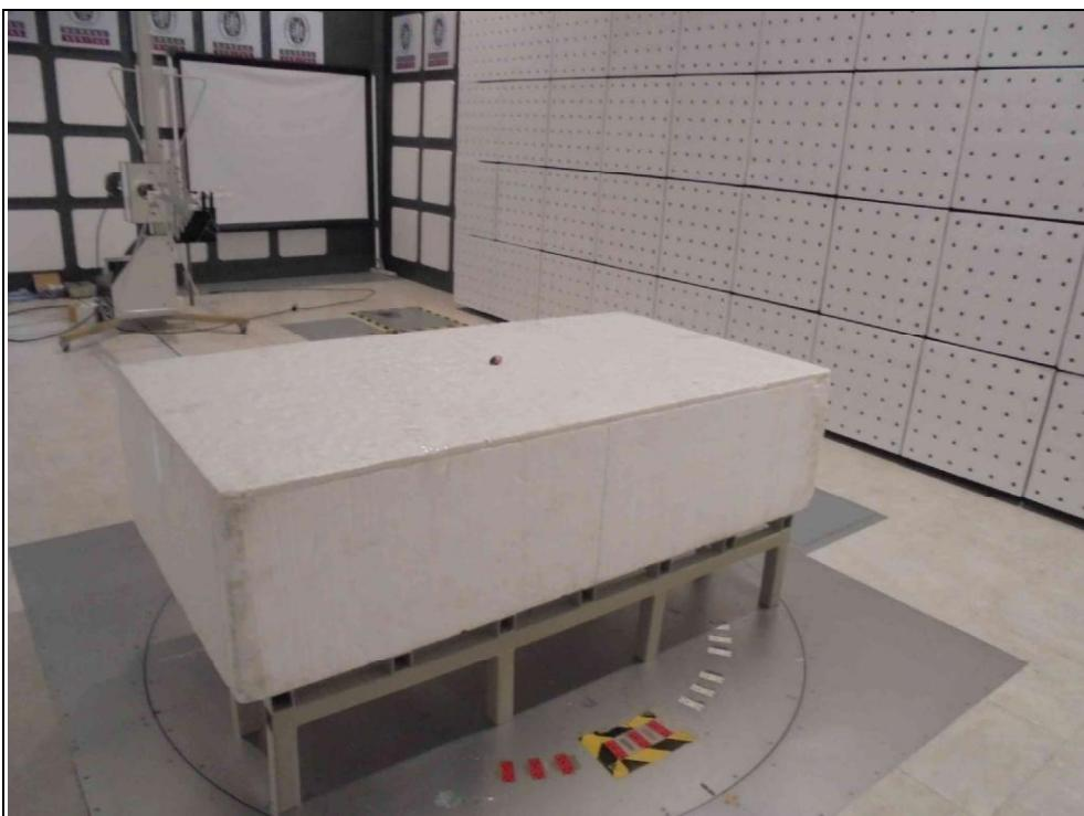
RADIATED EMISSION TEST - Mode A
