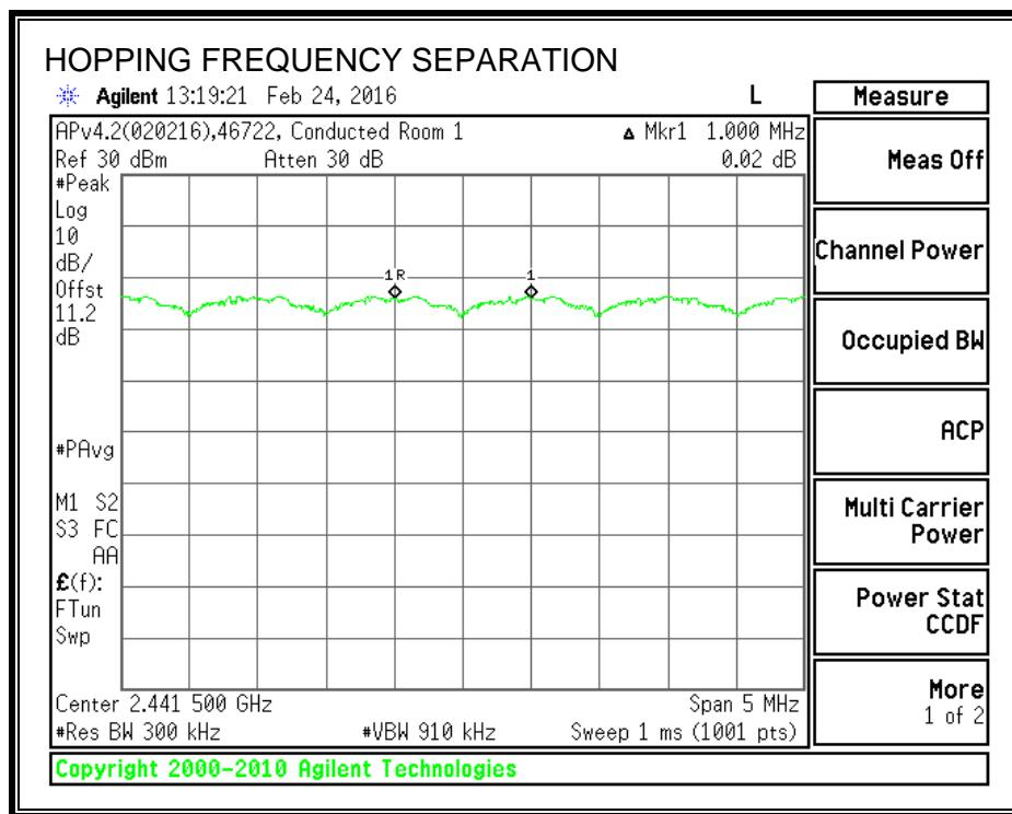
Note – The channel hopping separation of 1MHz is less than the 20 dB bandwidth (approx. 1.3 MHz). However, the output power is less than 125 mW and the channel separation is greater than 2/3 the 20 dB bandwidth (approx. 875 kHz).
