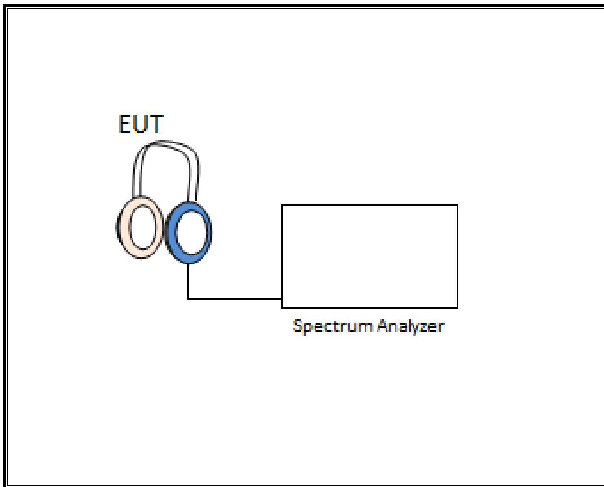
**SETUP DIAGRAM FOR RADIATED TESTS**
