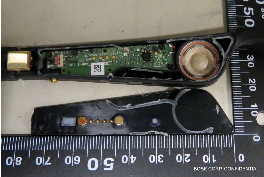
Internal product labelling – main PCB top
