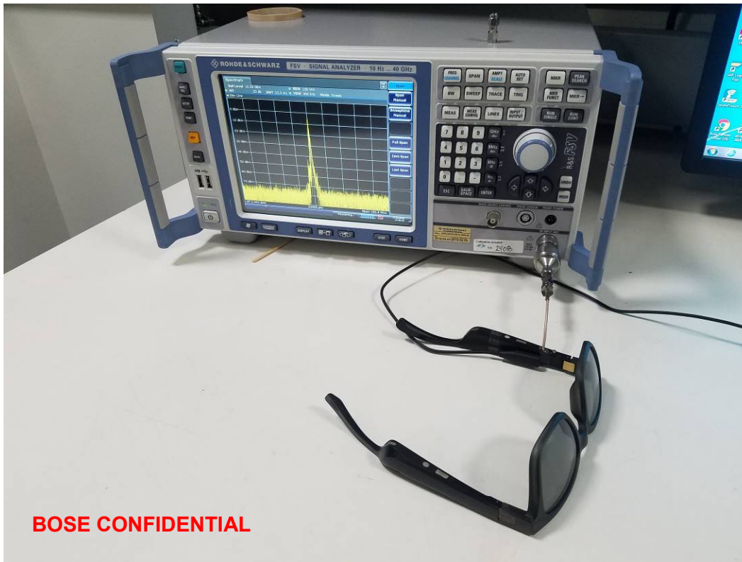
Antenna port conducted measurements
