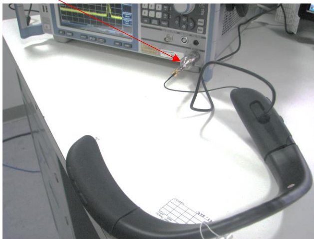
Setup with 2.4 GHz notch filter & 10 dB Pad
