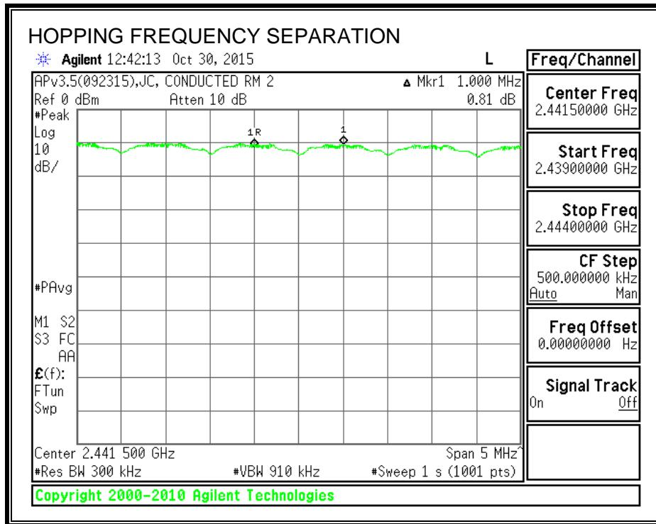
Note – The channel hopping separation of 1MHz is less than the 20 dB bandwidth (approx. 1.3 MHz). However, the output power is less than 125 mW and the channel separation is greater than 2/3 the 20 dB bandwidth (approx. 867 kHz).
