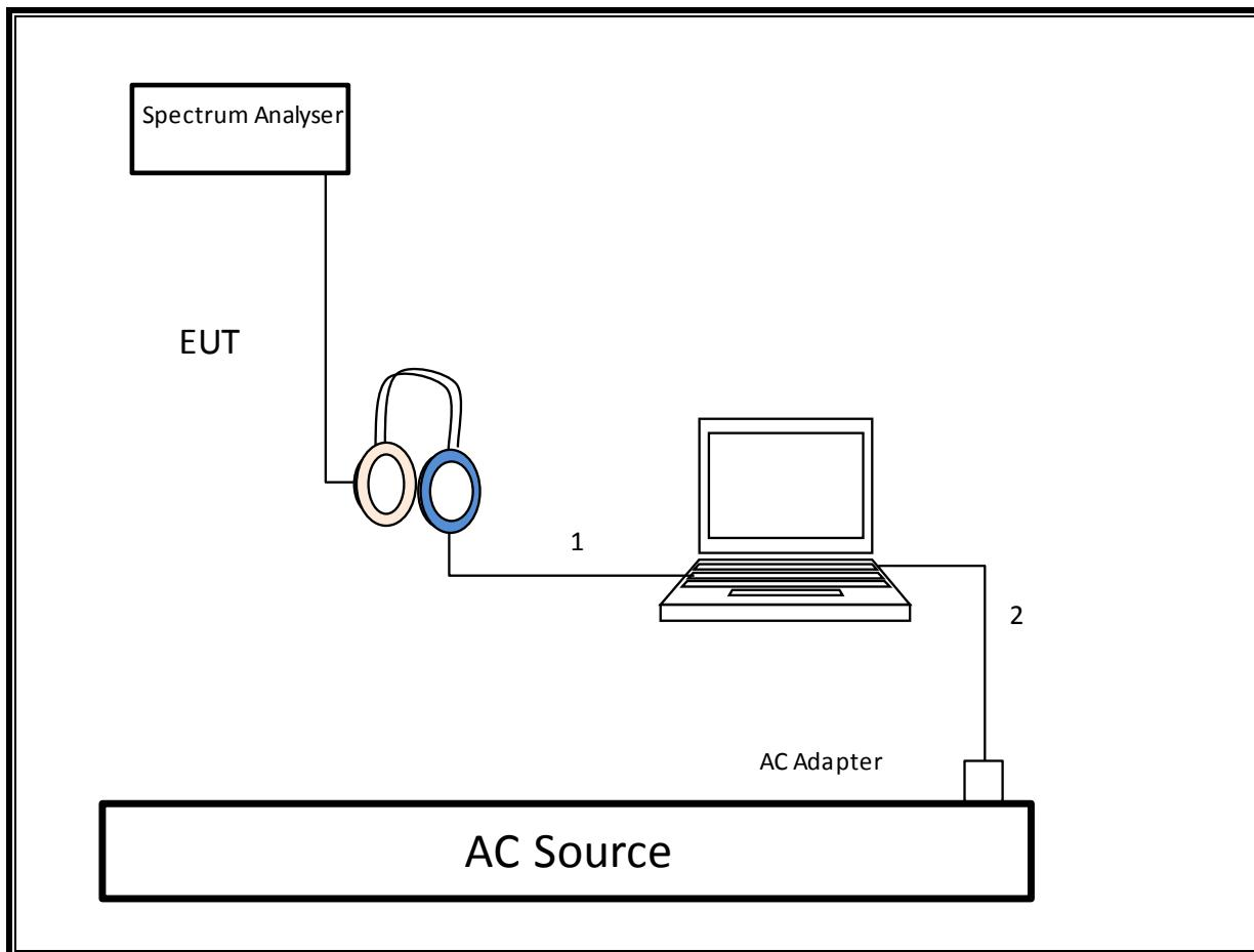
**SETUP DIAGRAM FOR RADIATED TESTS**
