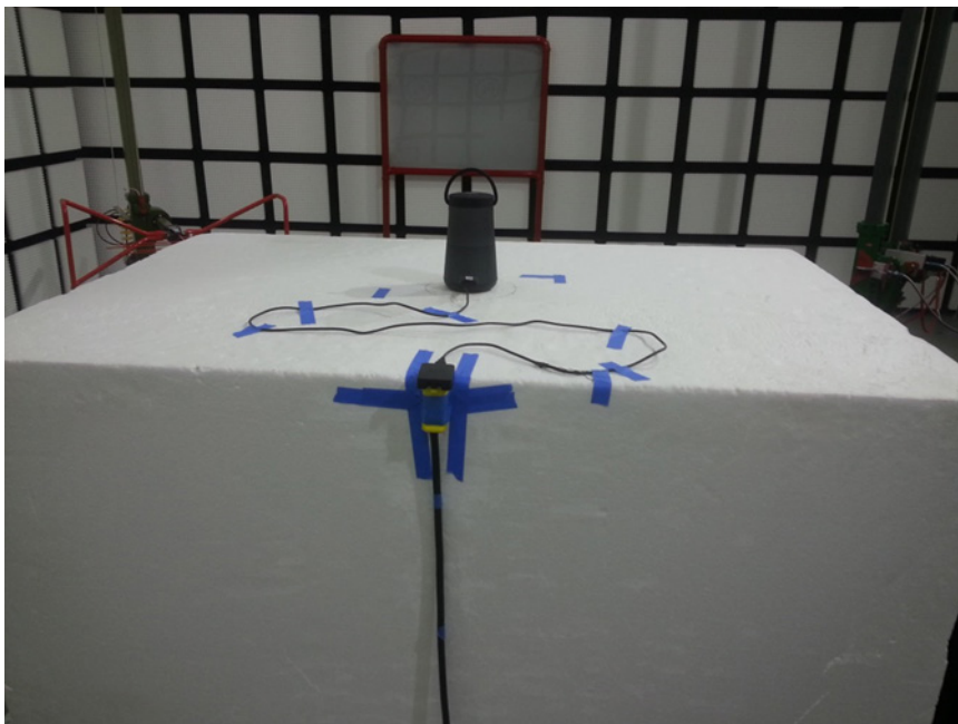
RADIATED SPURIOUS PHOTO – With Charger
