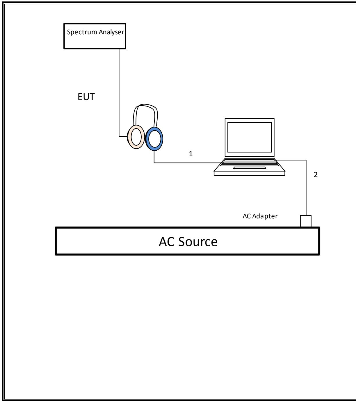
**SETUP DIAGRAM FOR RADIATED TESTS**
