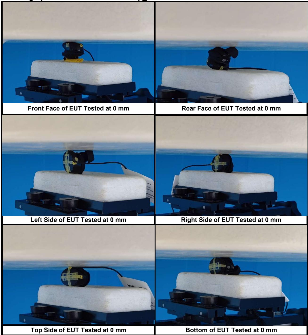
**<Photographs of Head SAR Test Setup\_Right Earbud>**
