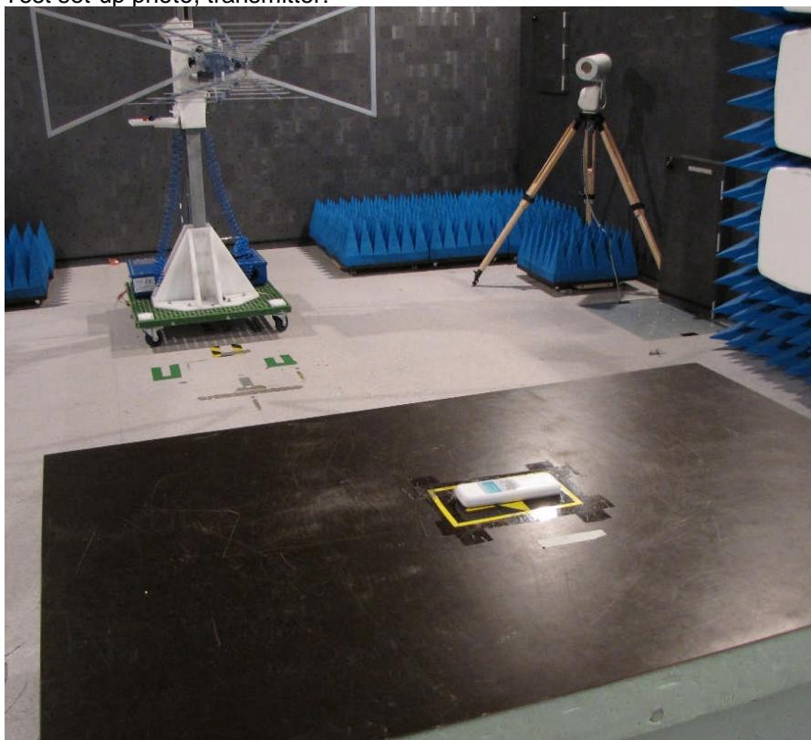
Test site: Big anechoic shielded chamber (1 – 10 GHz)
