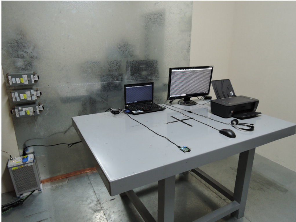
Photograph 6: Set-up for for Mains Conducted testing Front
