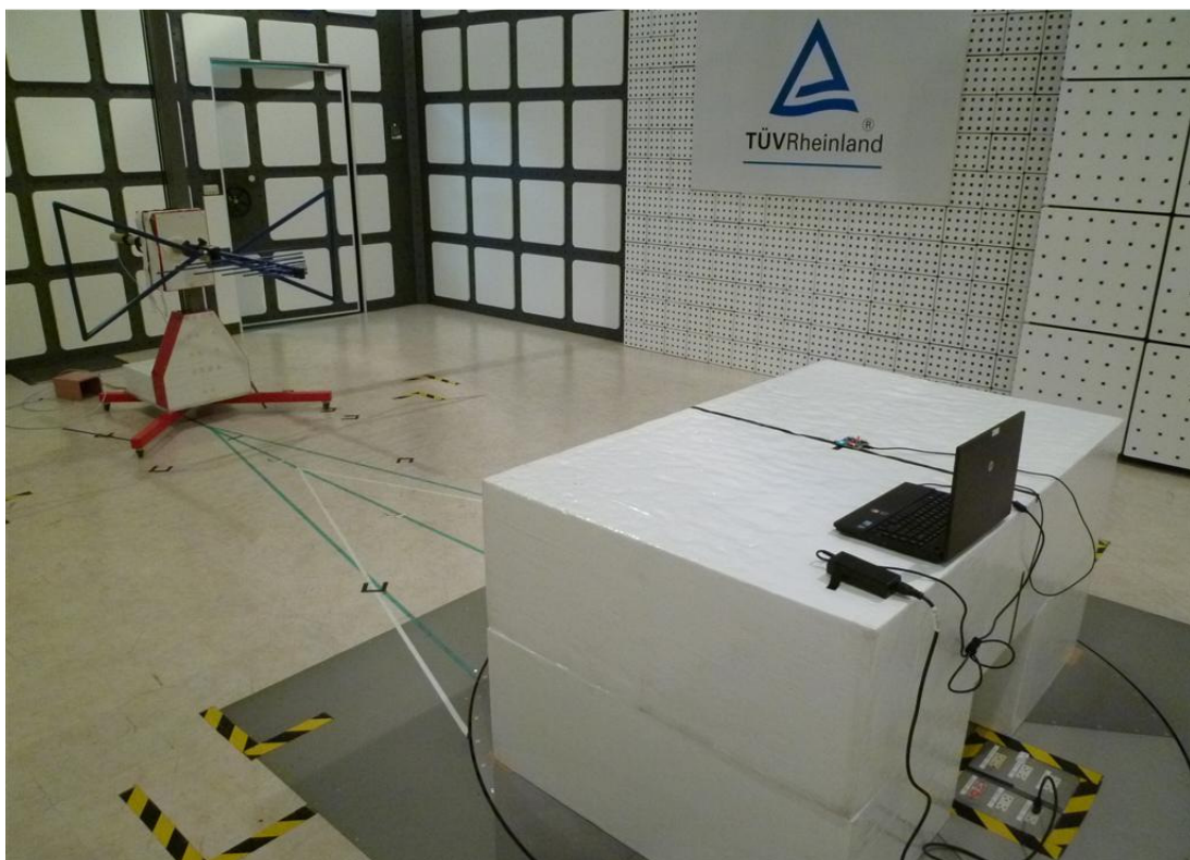
Photograph 2: Set-up for Spurious Emissions (Back View 1)
