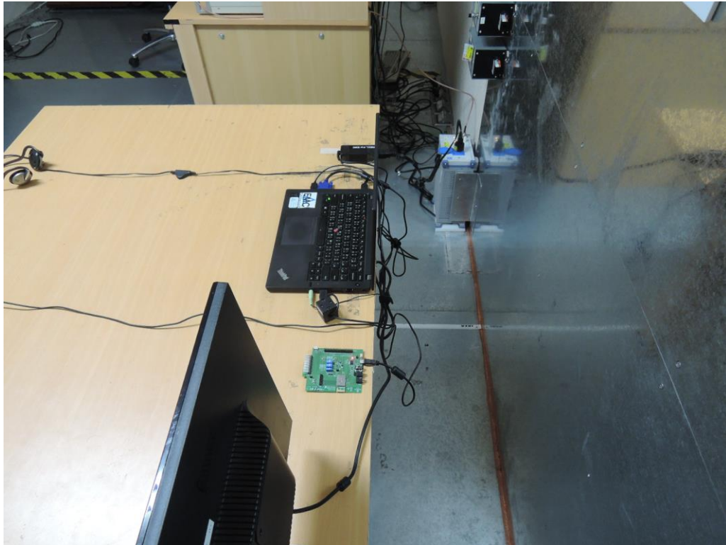
Photograph 5: Set-up for for Mains Conducted testing Back
