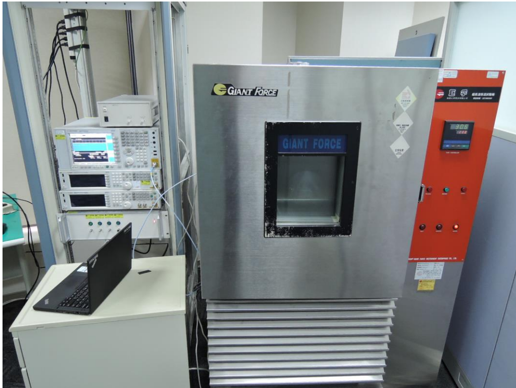
Photograph 4: Set-up for Conducted testing
