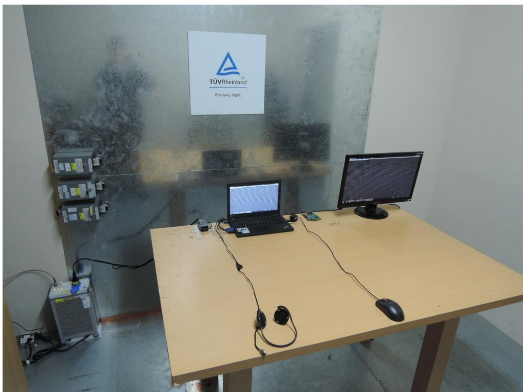
Photograph 6: Set-up for for Mains Conducted testing Front
