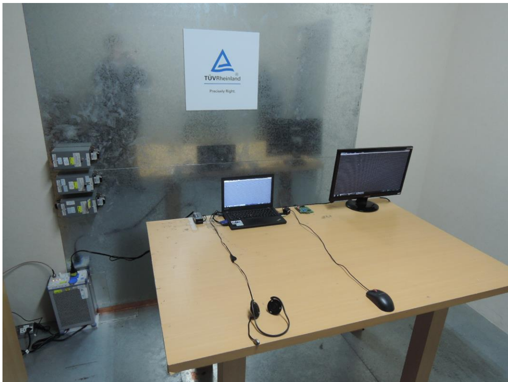
Photograph 6: Set-up for for Mains Conducted testing Front
