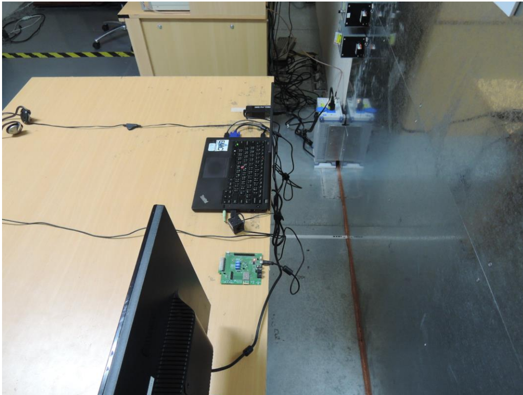
Photograph 6: Set-up for for Mains Conducted testing Front
