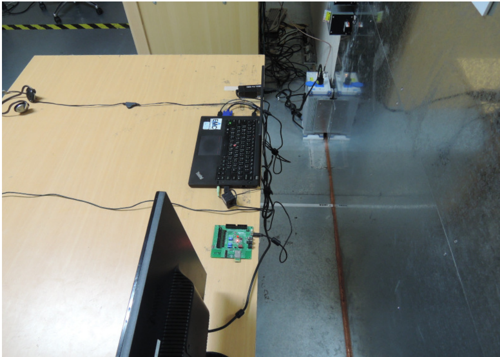
Photograph 5: Set-up for for Mains Conducted testing Back
