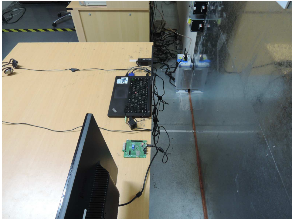
Photograph 5: Set-up for for Mains Conducted testing Back
