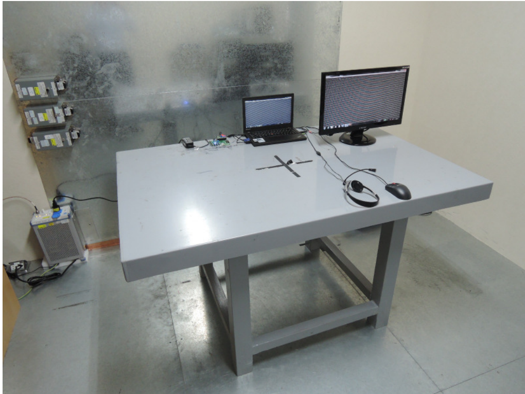
Photograph 8: Set-up for for Mains Conducted testing Front
