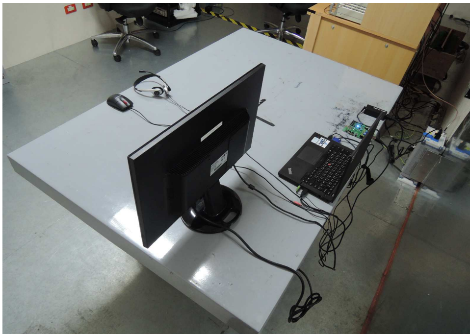
Photograph 7: Set-up for for Mains Conducted testing Back
