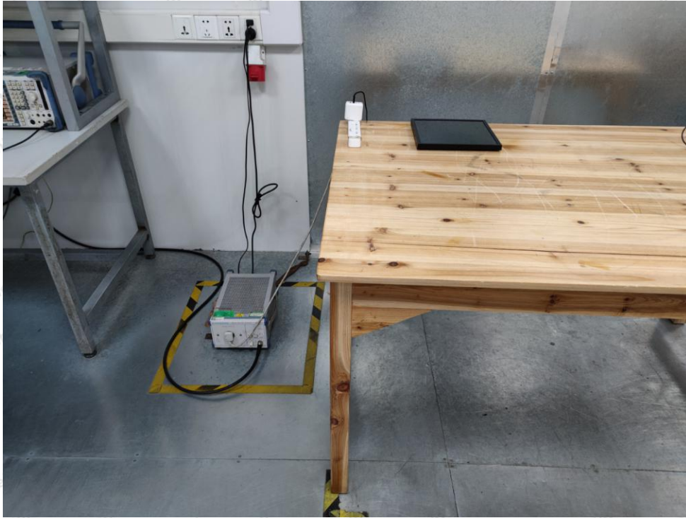
Photo of Power Line Conducted Emission Test
