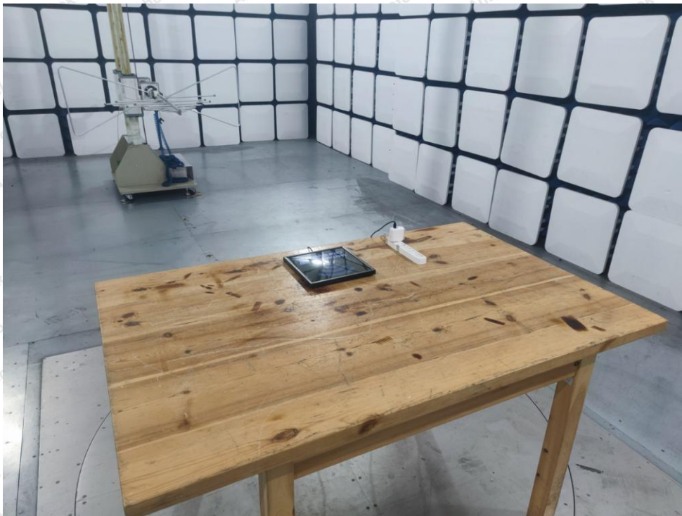
Photo of Radiation Emission Test
