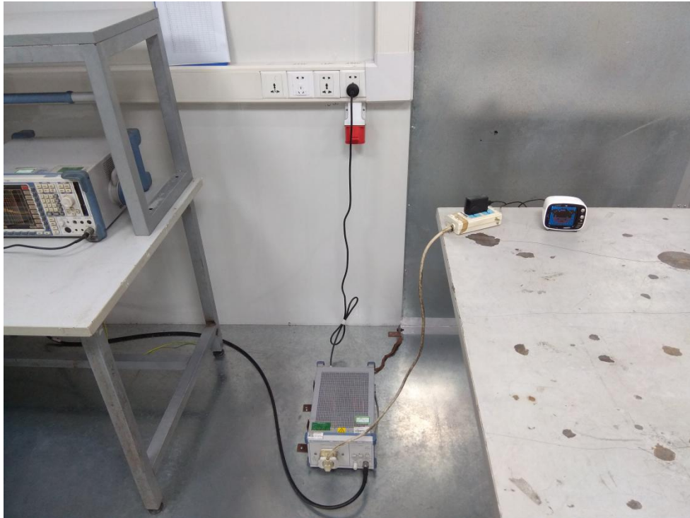
Photo of Conducted Emission Measurement
