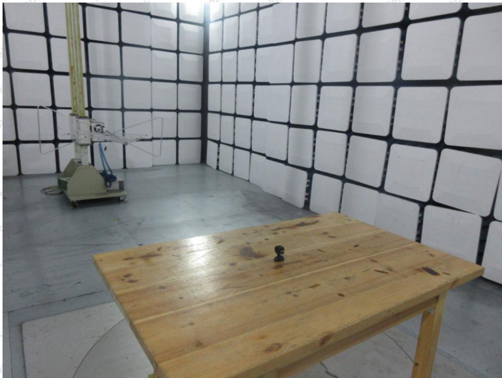
Photo of Radiation Emission Test
