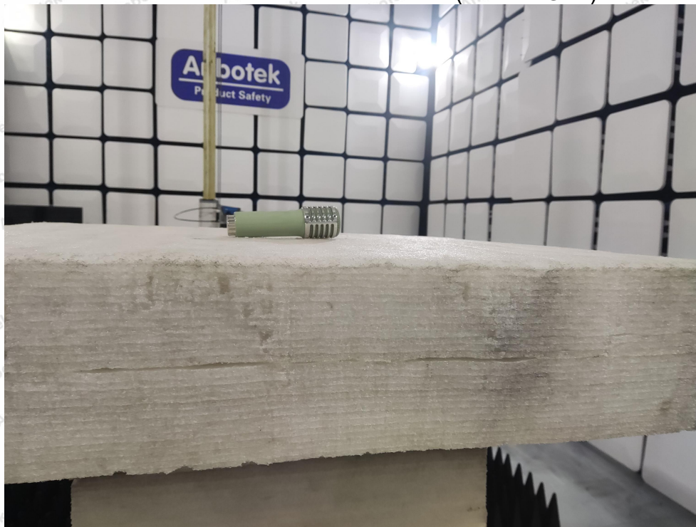
Photo of Radiation Emission Test (above 1GHz)
