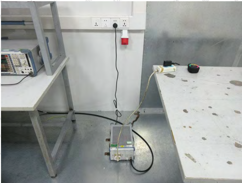
Photo of Conducted Emission Test
