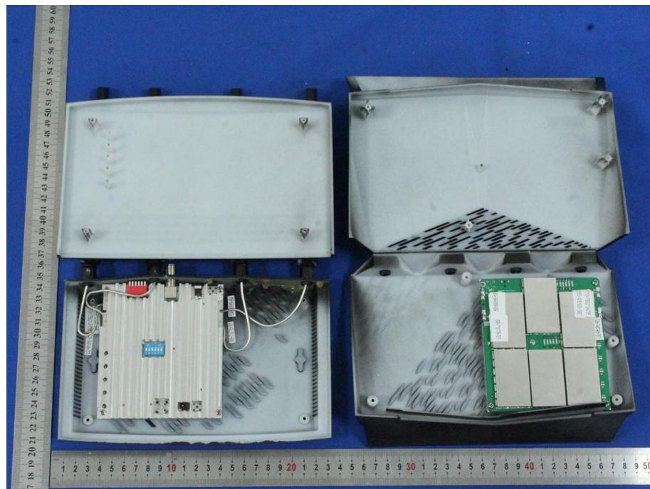
The circuits of the two samples are the same, only the positions of the donor port and the power port are different.
