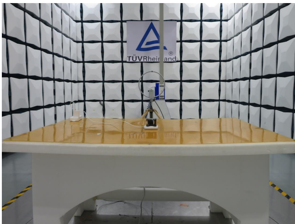
Photograph 1: Set-up photo for Radiated Spurious Emission, Below 30MHz
