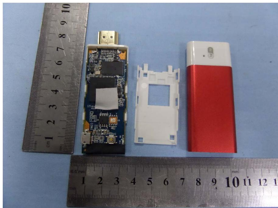
**Solder Board-Component View 1**
