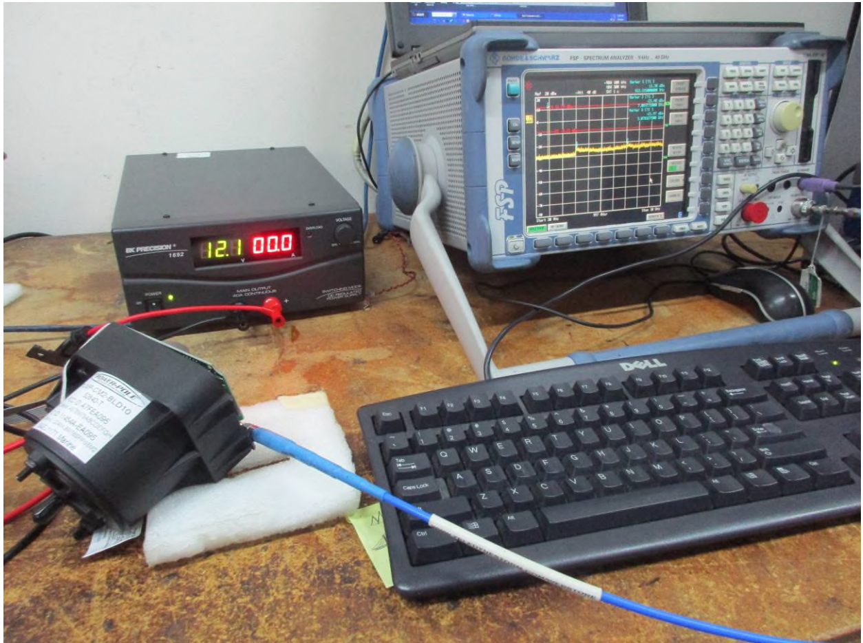
Figure 7: RF Conducted Emissions
